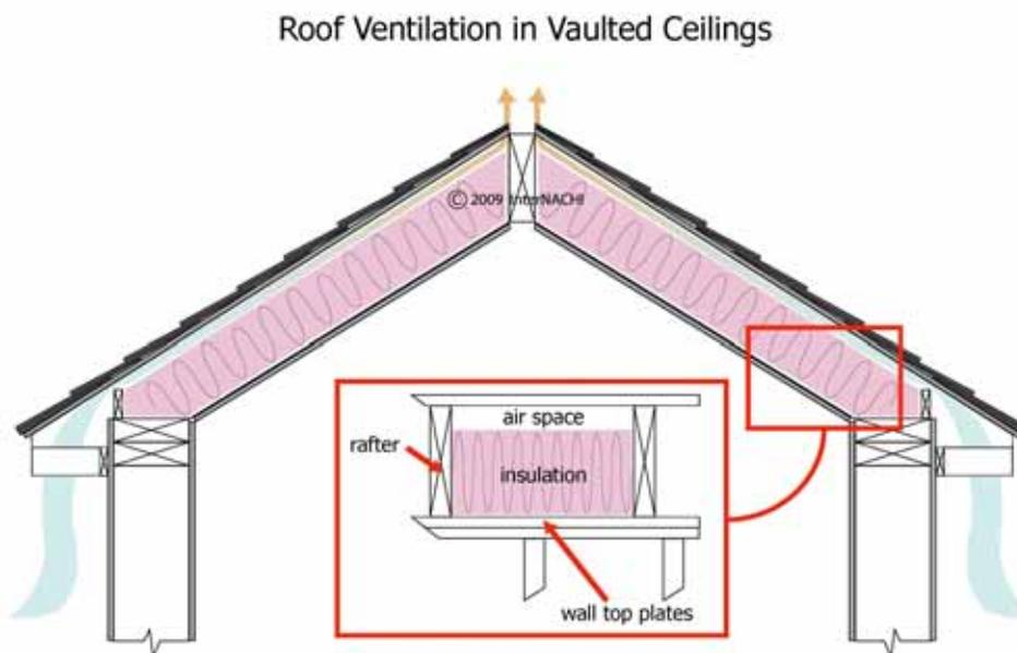
**Rafter vent trays.** To completely cover your attic floor with insulation out to the eaves you need to install rafter vents or trays (also called insulation baffles). Rafter vents
