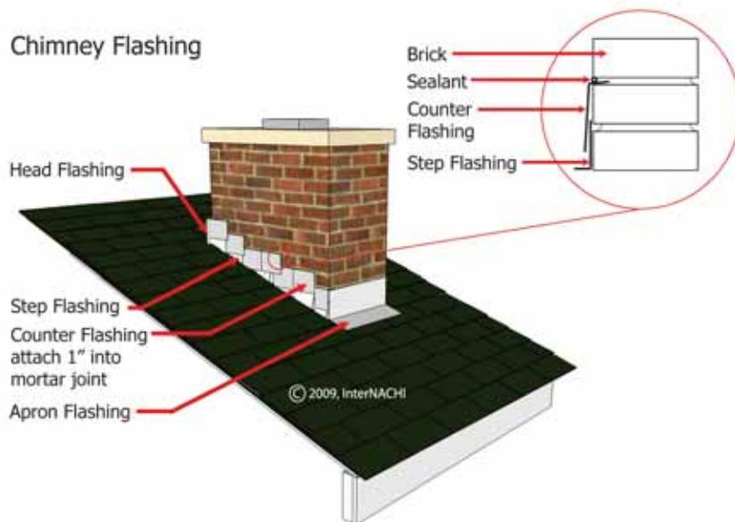
Most leaks occur around penetrations through the roof, such as at a chimney, plumbing vent, exhaust fan or skylight. Flashings and sealant joints around these penetrations can crack, fail and leak. Intersections of roof surfaces with walls are also a common leakage point.
